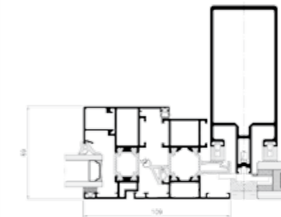
Active window in a curtain wall - cross-section
